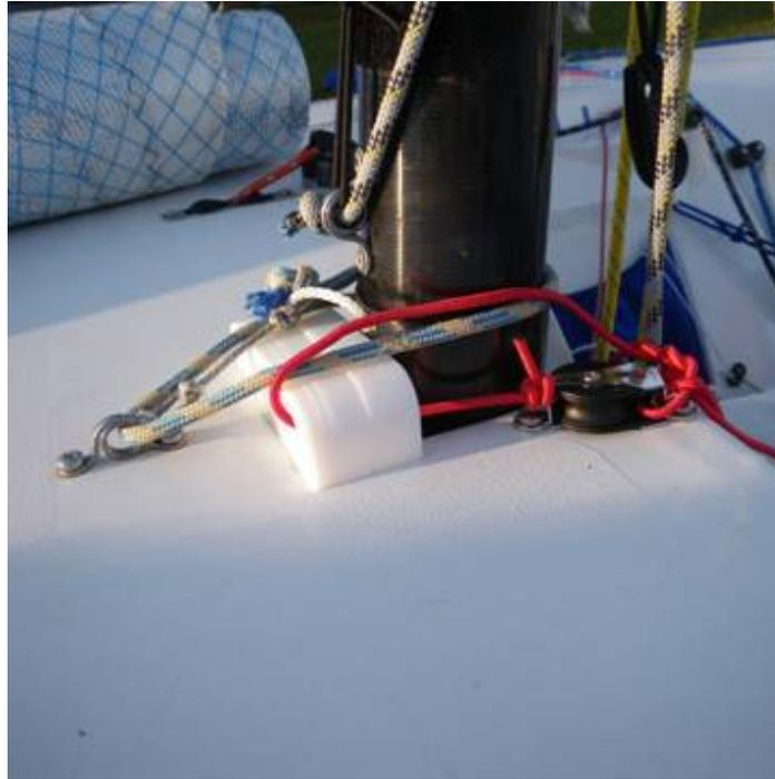
In this case we are using 1  $\frac{3}{4}$ " thick block, 1  $\frac{1}{2}$ " and 2  $\frac{1}{4}$ " thick blocks. This is what worked in this case to achieve 3  $\frac{1}{4}$ " of pre bend. The  $\frac{3}{4}$ " block has been filed out on the underside to accommodate the rake and spread the load on the front of the mast.
