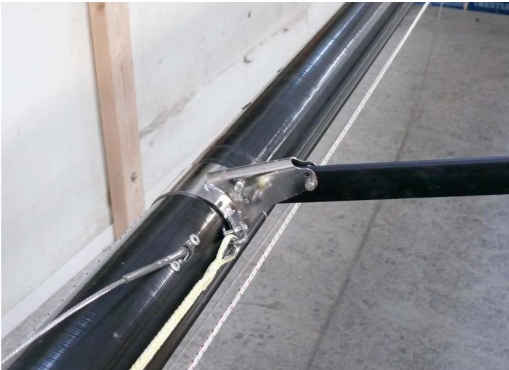
3. Once fitted correctly the excess bolt length should be cut off, and the ends filed smooth to prevent the spinnaker ripping on any jagged cut metal. It's always a good idea to wrap all of the potential snags the spinnaker may come in contact with using a little rigging or white electrical tape.
