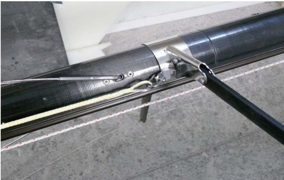
6. Measure the forestay BS to BS (Bearing Surface to Bearing Surface) and lock off the adjuster at 24ft 6". Undo the upper shrouds turnbuckles to maximum open.
