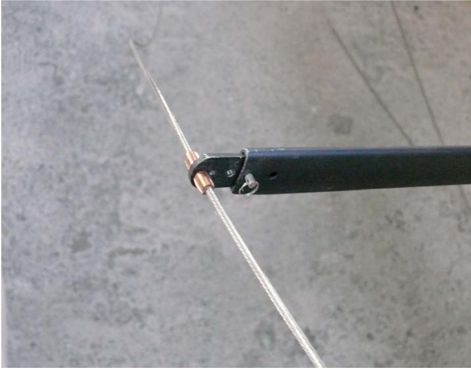
5. Take the dyneema keel hoist line and shackle it to the tang on the port side of the spreader bracket. Attach any wind indicators or similar to the head.
