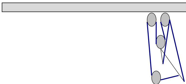
Diagram B. Split tail mainsheet arrangement attached to mid boat pad eyes
